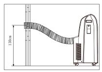
If duct is to be bent, please install it by considering following the dimensions.
