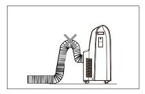
Wrong installation is shown in the following figure (If the pipe is bent too much, it could easily cause a malfunction.)
