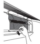
**4** Clean the large air filter/s with soapy water. Rinse with fresh water. Shake off excess water.
