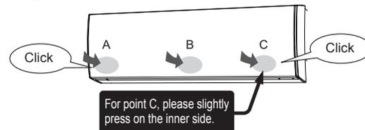
If the intake grille is not completely closed, the air-conditioner will not operate and the lamp will flash as shown below.
