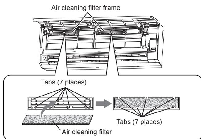
The new air cleaning filters can be attached to the right frame or the left frame.
