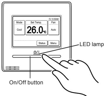
The LED lamp remains lit while the indoor unit is operating.
