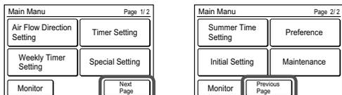
When the item to be set is touched, each setting screen is displayed. Refer to the description of each item for details. When each setting is complete or canceled, the display returns to this screen. When [Monitor] is touched, the display returns to the Monitor Mode Screen.
