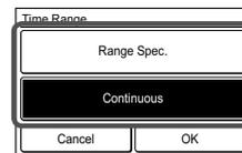
When the [OK] is touched, the display returns to the "Time Range Setting" screen. When the [Continuous] was selected, go to (14).
