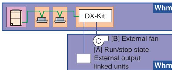
✗ The electricity meter is installed independently from the units [A] and [B].
