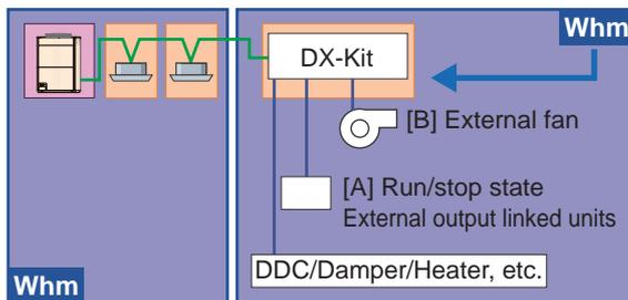
○ The electricity meter is installed so that [A], [B], and other units are included.
