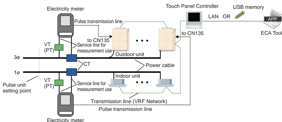
Pulses output with electricity meters specified in units of pulses are normalized (usually 1kWh/pulse) beforehand and then output.
