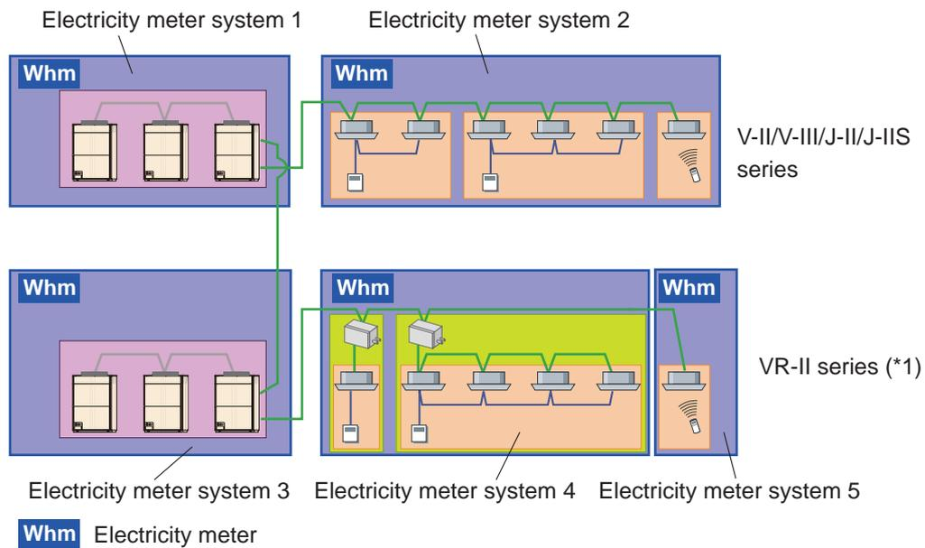
(\*1) In the VR-II series, Electricity Meter System can contain the RB units.
