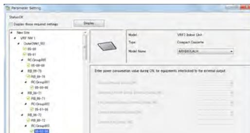
When a unit is ON/OFF linked and controlled by using the external output terminals on its PCB, entering the power at ON here can be taken into account for electricity charge apportionment calculation.
