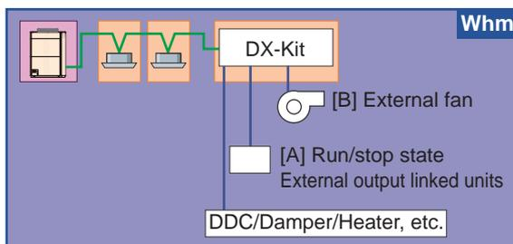
✗ The electricity meter is installed so that the units other than [A], [B] and indoor units are included.
