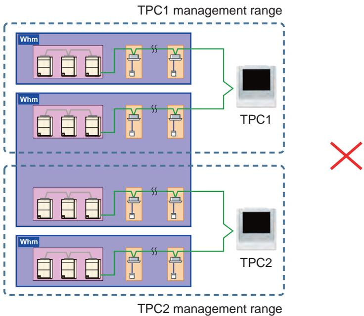
Connect the electricity meter that measures the units managed by the appropriate TPC to the electricity meter I/F belonging to the TPC main unit.
