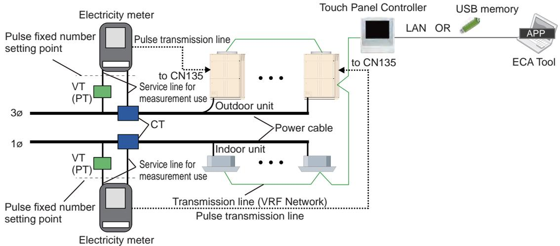
Consumed electricity values displayed by output pulses with an electricity meter specified in a fixed number of pulses must be corrected with the VT/CT ratio. In this case configure the following settings.
