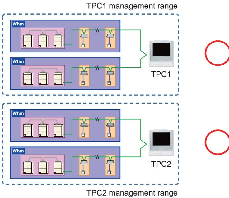
An electricity meter system spanning units managed by TPC cannot be created.
