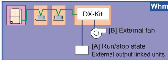
○ The electricity meter is installed so that the units [A] and [B] are included.
