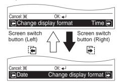
**NOTE:** These buttons are active only when any combinations of and the relevant screen names are displayed in the black field at the bottom of the screen.
