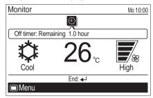
If multiple timers have been set, up/down arrows ▲ ▼ are displayed in the message balloon. To check the target timer function, press the [Cursor button (Up/Down)].
