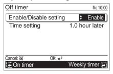
For [Time setting], adjust the time with the [Cursor button (Up/Down)], and press the [Enter button] to complete the setting.
