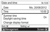
"Time" screen is displayed. Select the setting items (hour, min., or AM/PM) with the [Cursor button (Left/ Right)] and set with the [Cursor button (Up/Down)]. When setting the minutes, setting can be completed quickly if the button is pressed continuously.
