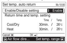
For [Return time and temp. setting], select operation mode with the [Cursor button (Up/Down)], and press the [Enter button]. Adjust the value with the [Cursor button (Up/Down)].
