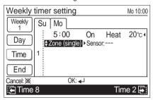
Select the room-temperature sensor with the [Cursor button (Up/Down)]. Then press the [Cursor button (Right)] to move the cursor to next setting item.
