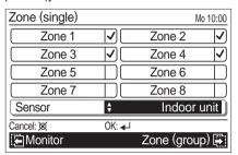
Each time you press the [Cursor button (Up/Down)], displayed sensor switches as follows.
