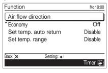
"Air flow direction" screen opens. In "Air flow direction" screen, adjustable airflow direction on the relevant indoor unit and its current specified movement are displayed.
