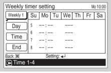
Press the [Enter button]. Then select [Weekly 1] or [Weekly 2] with the [Cursor button (Up/Down)], and press the [Enter button].
