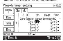
After you select all the applicable zones, press the [Enter button] to complete the individual setting of zone control.
