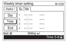
(2) Move the cursor between each pattern number with the [Cursor button (Up/Down)], and press the [Cursor button (Left/Right)] to set the time setting of On/Off timer, On/ Off, operating mode and temperature for each pattern.
