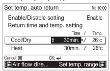
To complete the setting, press the [Enter button]. To return to the "Function" screen, press the [Cancel button].
