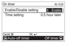
For [Time setting], adjust the time with the [Cursor button (Up/Down)], and press the [Enter button] to complete the setting.
