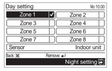
3 Select zone to be registered in the group with the [Cursor button]. When you press the [Enter button], a check mark is displayed.
