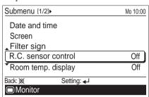
2 Select [On] or [Off] with the [Cursor button (Up/Down)], and press the [Enter button].
