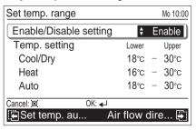
For [Temp. setting], select mode with the [Cursor button (Up/Down)] and press the [Enter button].
