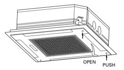
3. Hold down the hook at A and pull the filter out.
