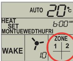
The display shows a heating system with 2 zones
