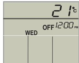
Adjusting the Time - Turn the Comfort Control OFF, open the door, press and hold the SET button for 3 seconds and go to Step 3
