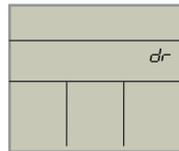
During a drain operation all buttons are in-operable and on restarting your cooler a delay will be experienced while the tank refills with fresh water.
