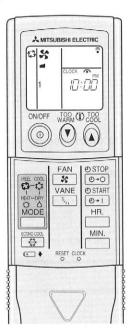
To change the AIR FLOW velocity, press the button.
