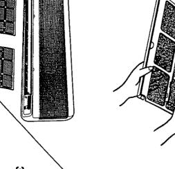
Put a sticker of sample colours (of dirt) at the lower part of the filter frame.
