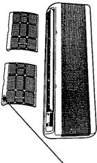
3. Be sure to set air filters back in place. Look at page 23 for replacing of air purifying filters.
