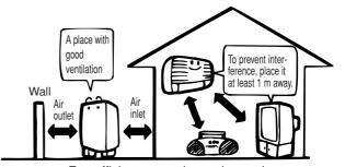
For efficient operation, take as large spaces around the unit as site allows.
