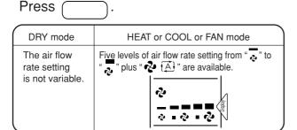
At smaller air flow rates, the cooling or heating effect is also smaller.
