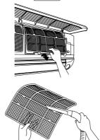
5 Set the air purifying filters and the air filters as they were and close the front grille.
