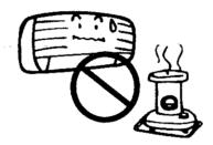
It may cause incomplete combustion or deformation of the unit from heat. Do not expose plants or animals directly to the air flow.
