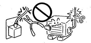
Applying a heavy weight, heat or tension on the power cord will damage it, causing electric shocks or fire.
