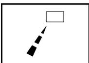
The AIR FLOW FLAP display stops swinging and the air flow direction is fixed (Fixed air flow direction setting).
