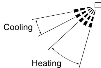
We recommend using the fan in the position listed above when fixing the fan direction.
