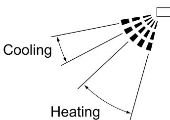
We recommend using the fan in the position listed above when fixing the fan direction.
