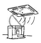
Never place nor use any inflammable sprays near the air conditioner, since such sprays could cause a fire.
