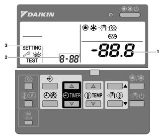
1 Press the button for a minimum of 5 seconds to enter FIELD SET MODE.
