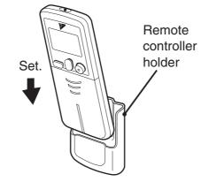
• To remove, pull it upwards.
