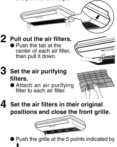
Operation without air filters may result in troubles as dust will accumulate inside the indoor unit.
