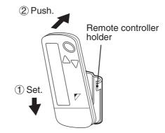
■ To remove, pull it upwards.
