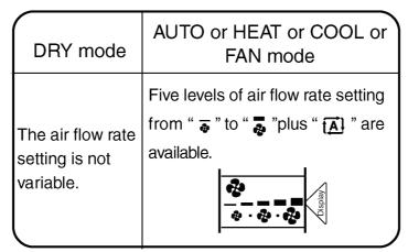
At smaller air flow rates, the cooling effect is also smaller.
