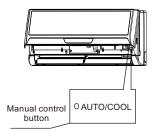
**NOTE:** The unit must be turned off before operating the manual control button. If the unit is operational, continue pressing the manual control button until the unit is off. ① Open and lift the front panel up to an angle
