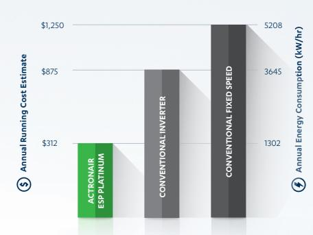
Based on electricity price of 24c per kW/H and the cooling energy consumption, this translates to a saving of up to \$900 per annum compared to conventional fixed speed systems.
